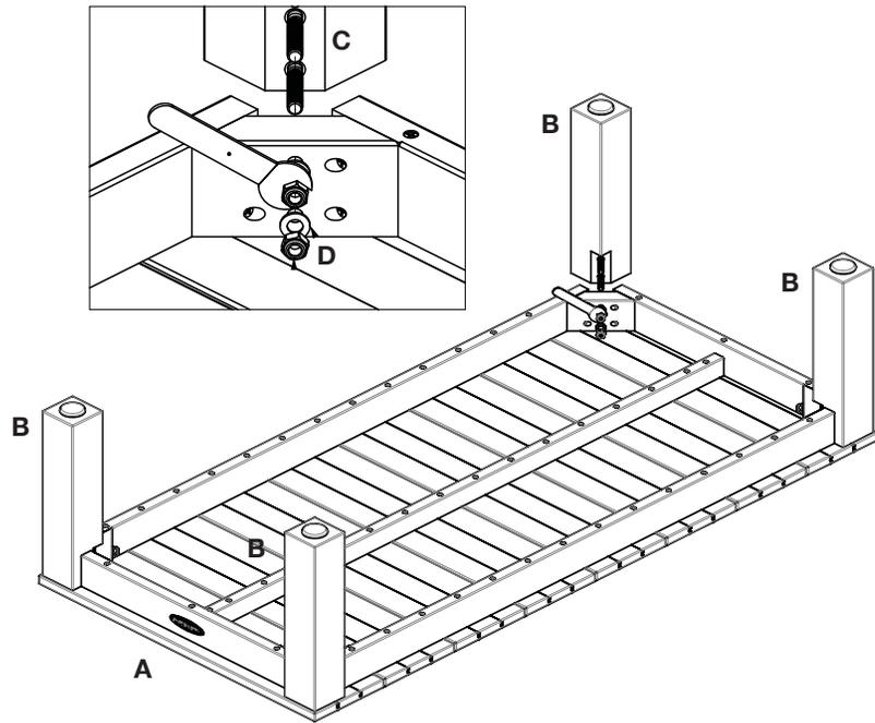
**1.** Carefully place the Table Top (A) face down on a protected surface. Attach Legs (B) to top of table by inserting threaded bolts at Leg top through holes at the corners of Table Top. Secure the Leg with Flat Washer (C) and Lock Nut (D) and tighten fully using Wrench provided.
