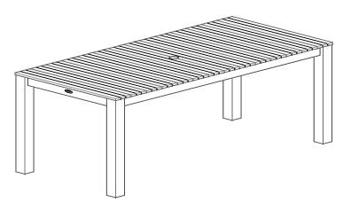
2. Ensure all fittings on legs are fully tightened before turning the table upright.
