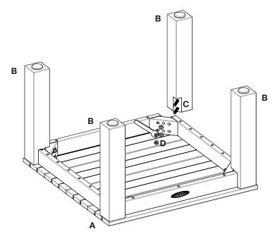
1. Carefully place the Table Top (A) face down on a protected surface. Attach Legs (B) to top of table by inserting threaded bolts at Leg top through holes at the corners of Table Top. Secure the Leg with Flat Washer (C) and Lock Nut (D) and tighten fully using Wrench provided.
